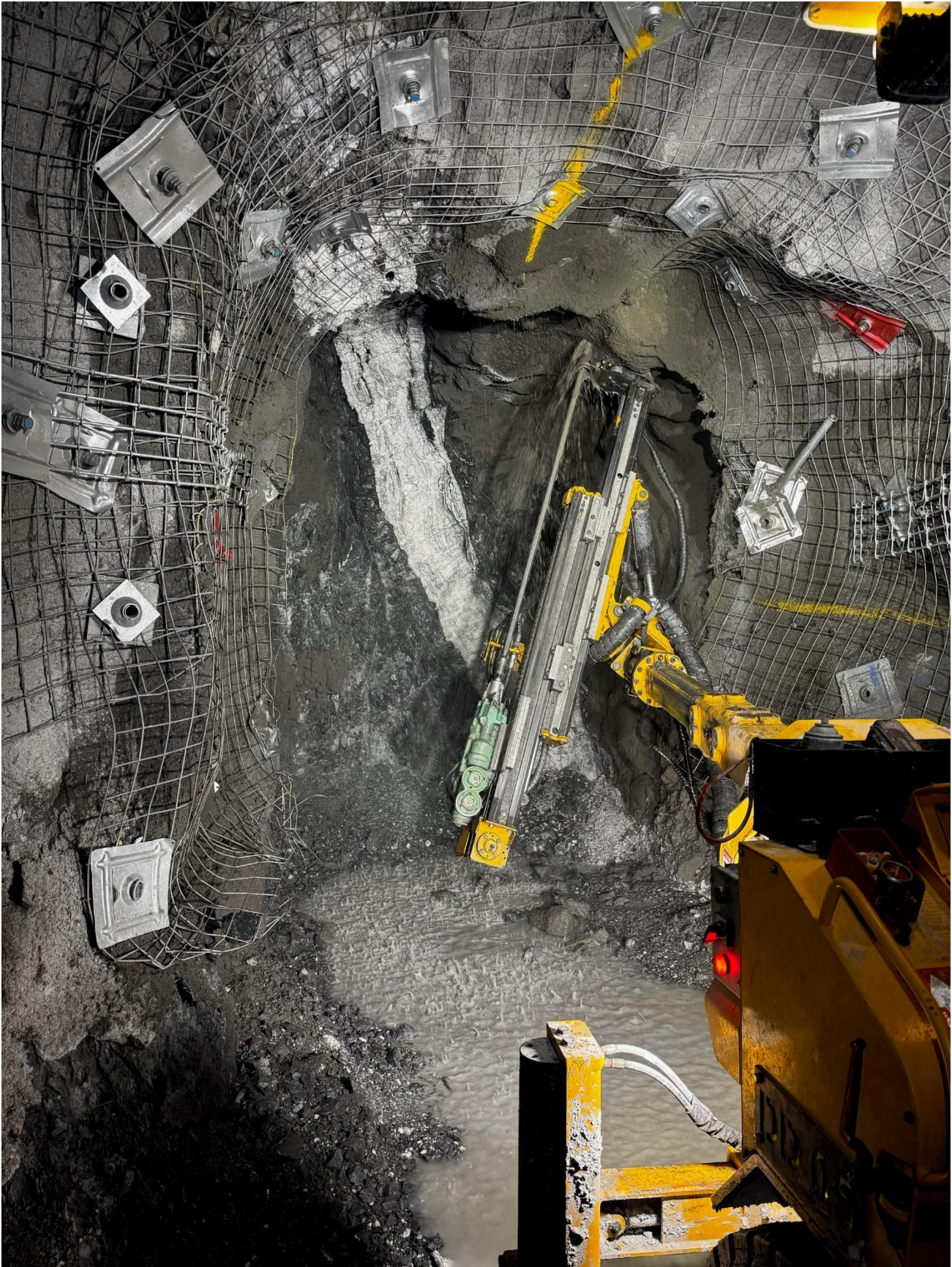
Photo – Single boom jumbo accessing the Birthday reef in ore drive
