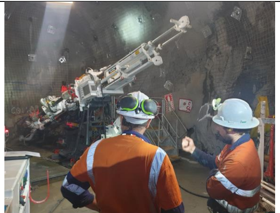
Photo 1 – Diamond drilling operations
