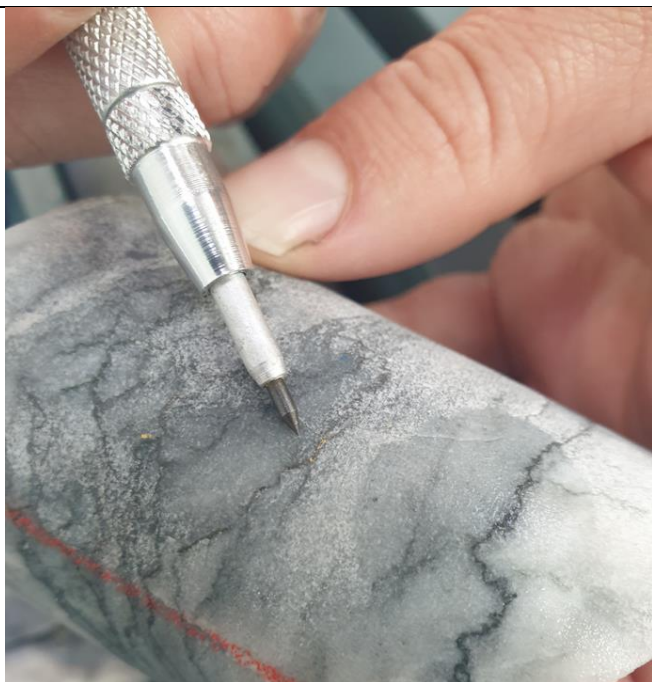
Photo 2 - Visible gold in drill core
