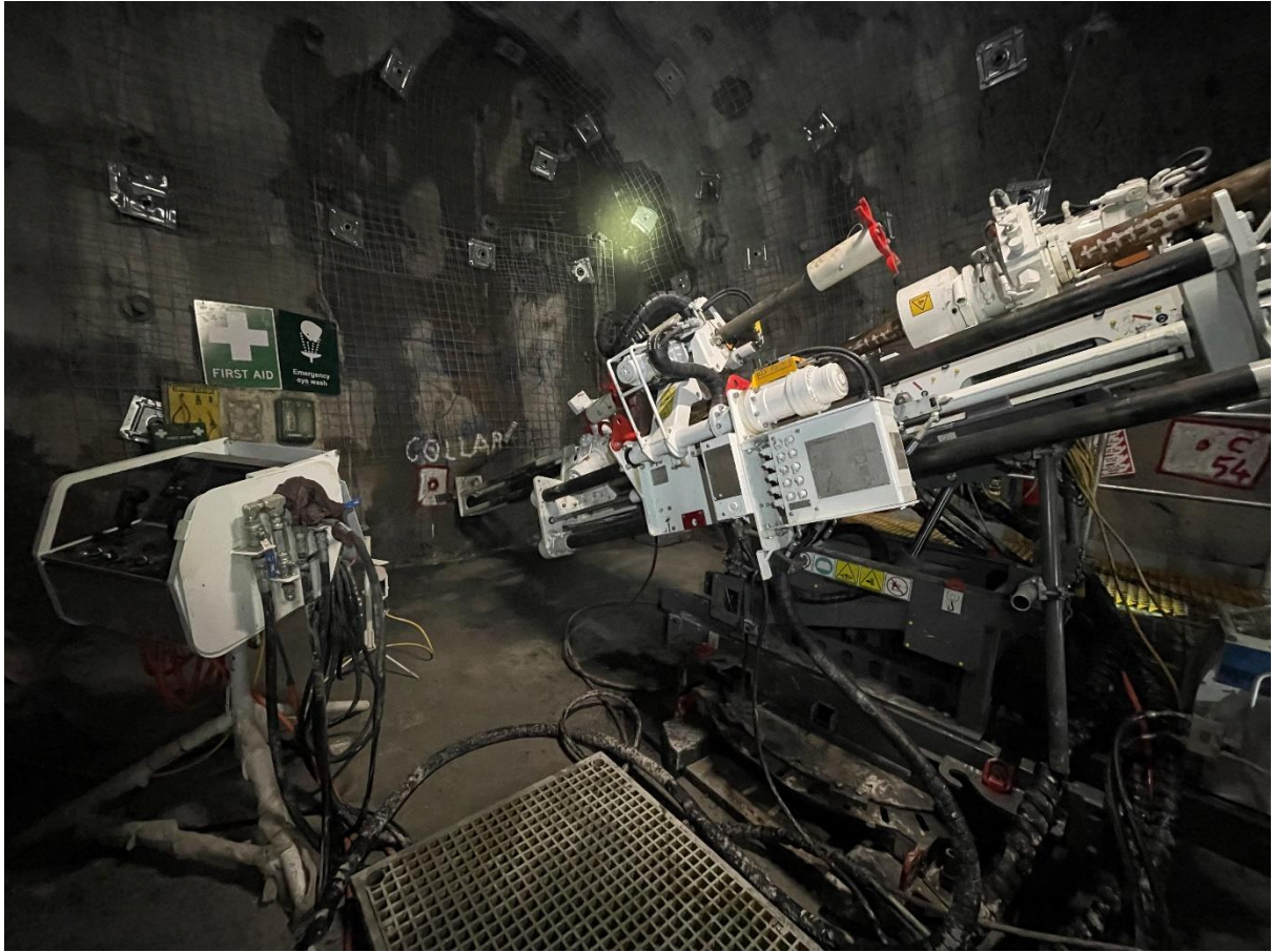
Diamond Drill Rig underground at Snowy River
