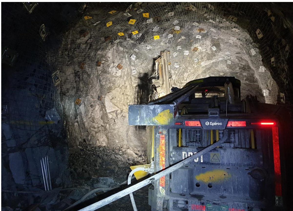
Epiroc M2D Jumbo working in the Main Decline
